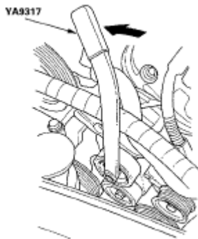
Fig. 15: Moving Auto-Tensioner Within Its Limit Using Belt Tension Release Tool Courtesy of AMERICAN HONDA MOTOR CO., INC.
